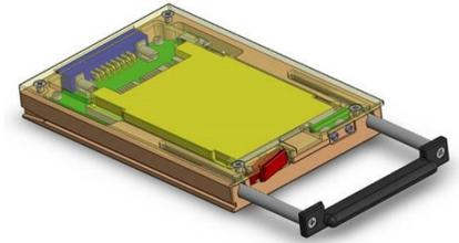
*Avionics Ejectable Solid-State Drive*
